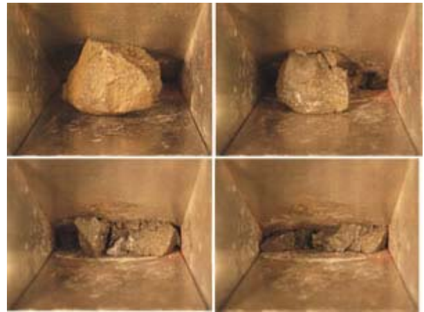
Looking down on the jaws of the Mars Rock Crusher, we see a magnetite rock get crushed into smaller and smaller particles.
